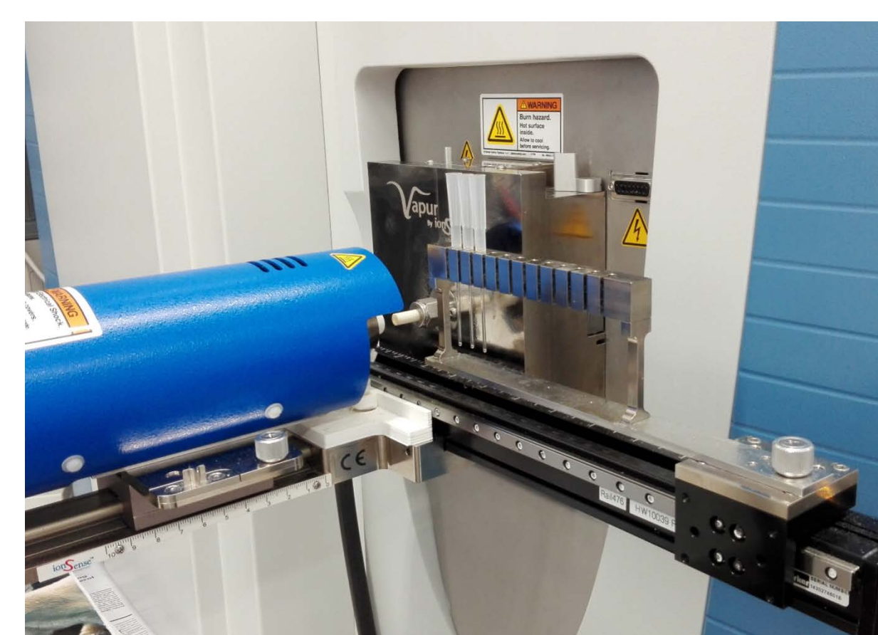
Fig.1 DART ion source with ORBITRAP inlet
